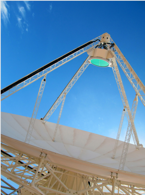
► The first ASKAP antenna to be installed with a PAF, an innovative receiver with many separate, simultaneous beams that will provide ASKAP with a wide field-of-view, allowing it to map the sky more quickly than alternative technologies. Credit: Barry Turner, CSIRO.
